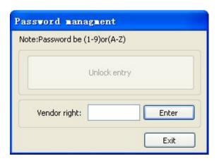
If the system is unencrypted, "Unlock entry" button will be in prohibited use state. Input the vendor password at "Vendor right", and then click "Enter" button to enter the password management interface.
